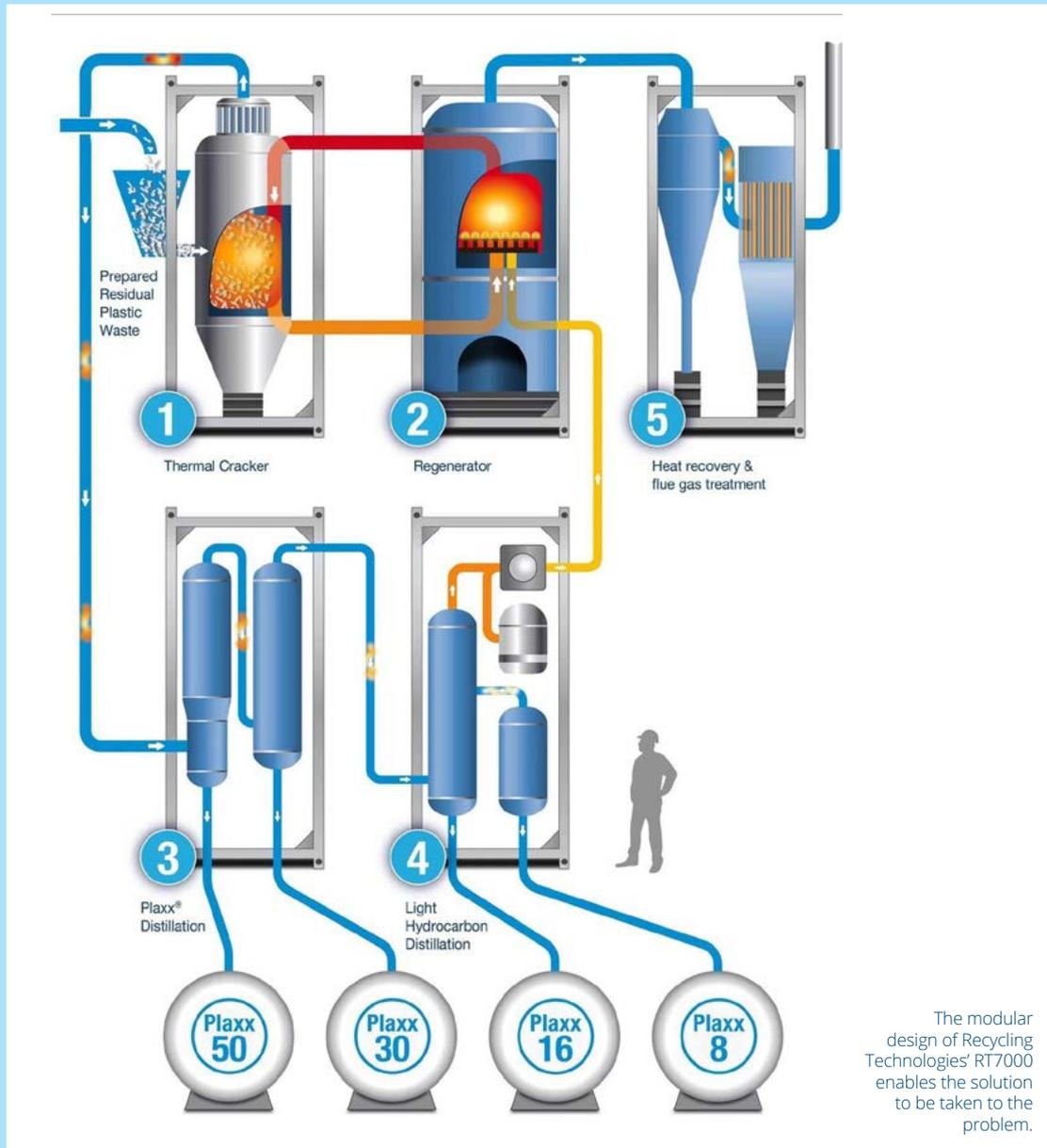
The modular design of Recycling Technologies' RT7000 enables the solution to be taken to the problem.
